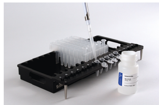
Figure 1. Setup and configuration of deck trays. Elution Buffer is added to the elution tubes as shown. Plungers are in well #8 of the cartridge. Deck tray shown is from the Maxwell ® RSC Instrument (Cat.# AS4500).
