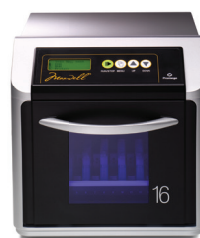
Figure 4.11. The Maxwell® 16 Instrument uses paramagnetic-particle technology to extract DNA, RNA or protein from up to 16 samples in less than 45 minutes. The paramagnetic particles and reagents are supplied in prefilled cartridges for faster separations with less hands-on time.
